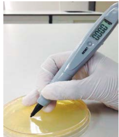
Figure 7. Colony counter (Fisher Scientific brand, model F22 0360/10R) used to measure the total colony forming units
